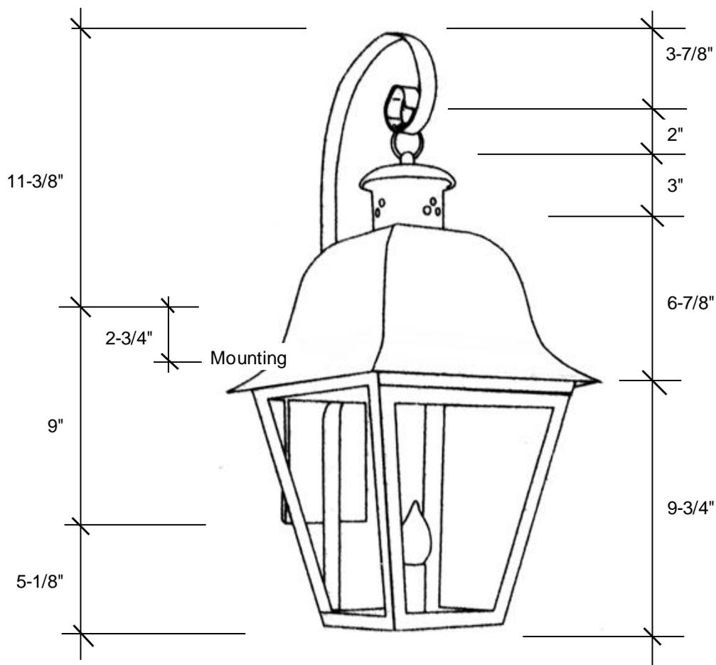
This fixture comes standard with clear glass, but seeded is available, and has (1) edison base socket that is listed for 60W with an option of (4) candleabra sockets that is listed for 40W each.
