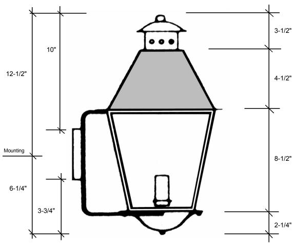
This fixture comes standard with clear glass, but seeded is available, and has a (1) edison socket that is listed for 60W with an option of a 4-light cluster that is listed for 40W each socket.
