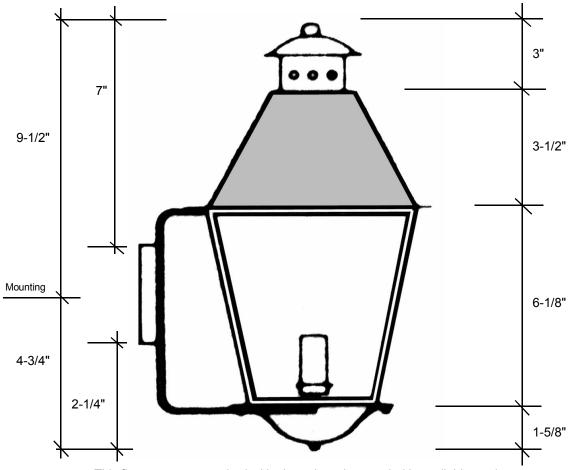
This fixture comes standard with clear glass, but seeded is available, and has a (1) edison socket that is listed for 60W with an option of a 2-light cluster that is listed for 60W each socket.
