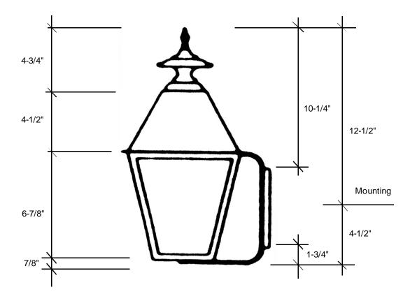
This fixture comes standard with clear glass and (1) medium base socket. A 4-light cluster, seeded glass and side scrolls are also available on this fixture. The 1-light is U.L. listed for 60W and the 4-light is listed for 40W each socket.
