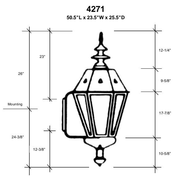
This fixture comes standard with clear glass, but seedy is available, and has (1) edison socket that is U.L. listed for 60W with an option of a 3-light cluster that is U.L. listed for 60W each socket.
