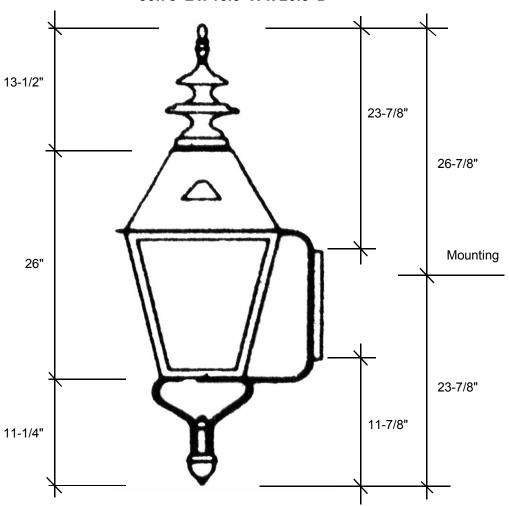
This fixture comes standard with clear glass and (1) medium base socket. A 4-light cluster, seeded glass and side scrolls are also available on this fixture. The 1-light is U.L. listed for 60W and the 4-light is listed for 40W each socket.
