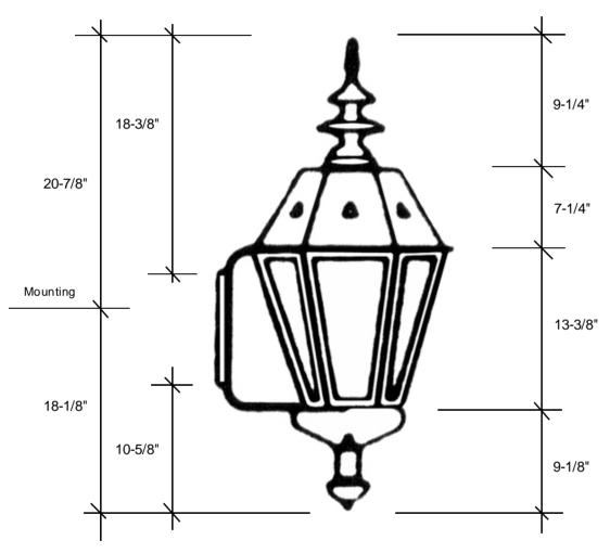
This fixture comes standard with clear glass, but seedy is available, and has (1) edison socket that is U.L. listed for 60W with an option of a 3-light cluster that is U.L. listed for 60W each socket.
