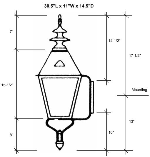
This fixture comes standard with clear glass and (1) medium base socket. A 4-light cluster, seeded glass and side scrolls are also available on this fixture. The 1-light is U.L. listed for 60W and the 4-light is listed for 40W each socket.
