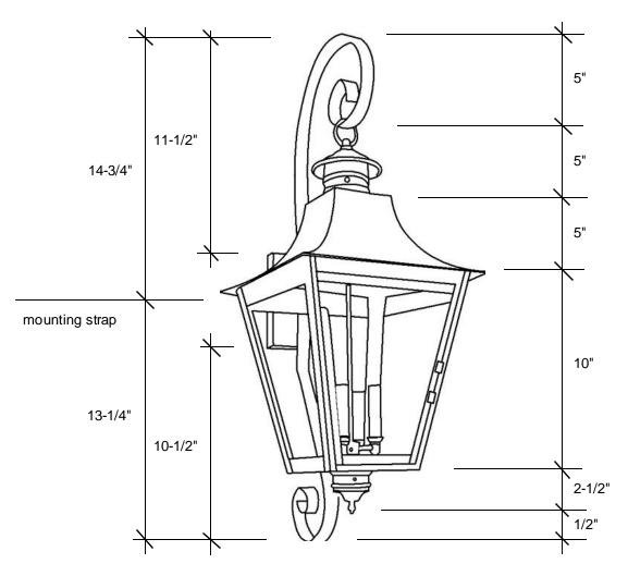
This fixture comes standard with clear glass, but seedy is available, and has (2) candelabra sockets that are listed for 60W each, with an option of a 4-light cluster that is listed for 40W per socket.
