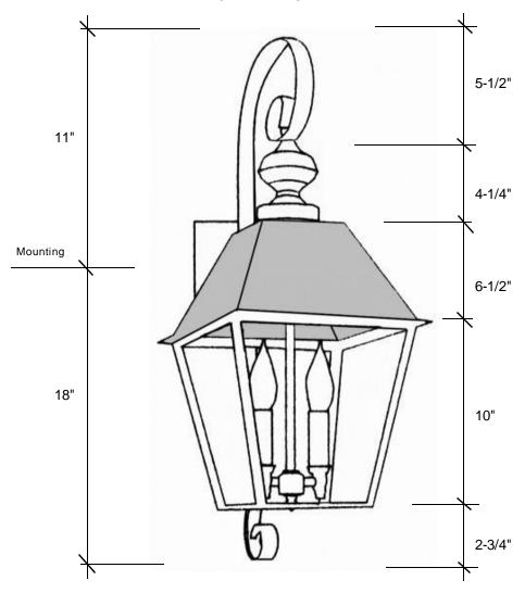
This fixture comes standard with clear glass, but seedy is available, and has (2) candelabra sockets that are listed for 60W each, with an option of a 4-light cluster listed for 40W per socket.
