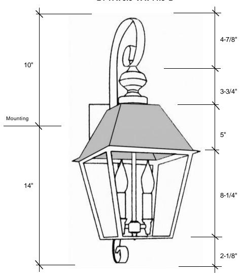
This fixture comes standard with clear glass, but seedy is available, and has (2) candelabra sockets that are listed for 60W each, with an option of a 4-light cluster listed for 40W per socket.
