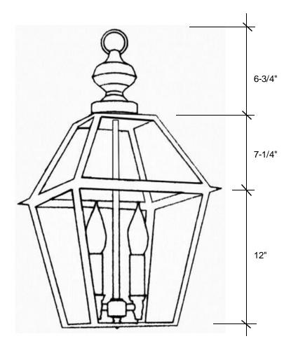
This fixture comes standard with clear glass, but seeded is available, and has (2) candelabra base sockets that are listed for 60W, with an option of a (4) light candelabra cluster listed for 40W per socket. 3' chain standard.
