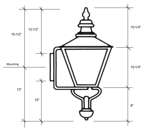
This fixture comes standard with clear glass, but seedy is available, and has (1) edison socket that is U.L. listed for 60W with an option of a 4-light cluster that is U.L. listed for 40W each socket.
