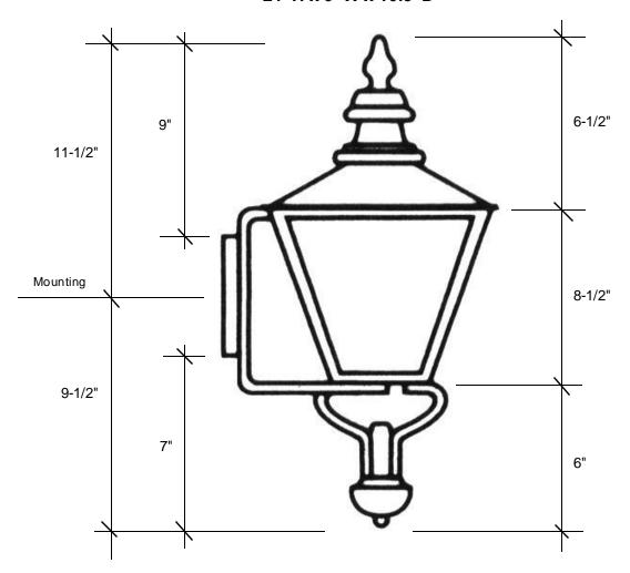
This fixture comes standard with clear glass, but seedy is available, and has (1) edison socket that is U.L. listed for 60W with an option of a 2-light cluster that is U.L. listed for 60W each socket.
