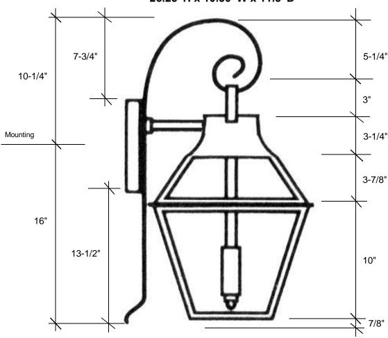
This fixture comes standard with clear glass, but seeded is available, and has a 2-light candelabra cluster that is U.L. listed for 60W each socket, with an option of a 4-light cluster that is UL listed for 40W per socket.
