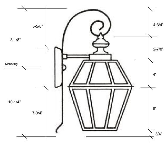
This fixture comes standard with clear glass, but seeded is available, and has a 2-light candelabra cluster that is U.L. listed for 60W each socket.
