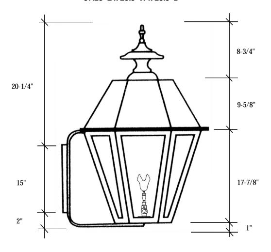
This fixture is available with clear tempered glass only and is UL listed for natural gas, with an option of propane. The fixture has a manual on/off valve with a maple leaf design and has a BTU rating of 3011.
