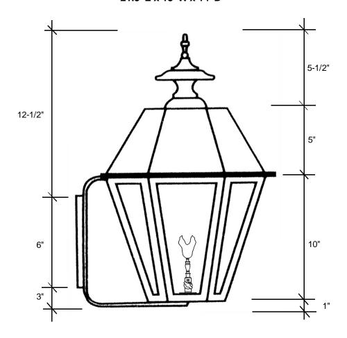
This fixture is available with clear tempered glass only and is UL listed for natural gas, with an option of propane. The fixture has a manual on/off valve with a maple leaf design and has a BTU rating of 3011. Electronic starters are not available.
