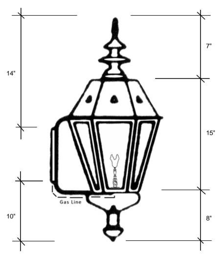
This fixture is available with clear tempered glass only and is UL listed for natural gas, with an option of propane. The fixture has a manual on/off valve with a maple leaf design and has a BTU rating of 3011.
