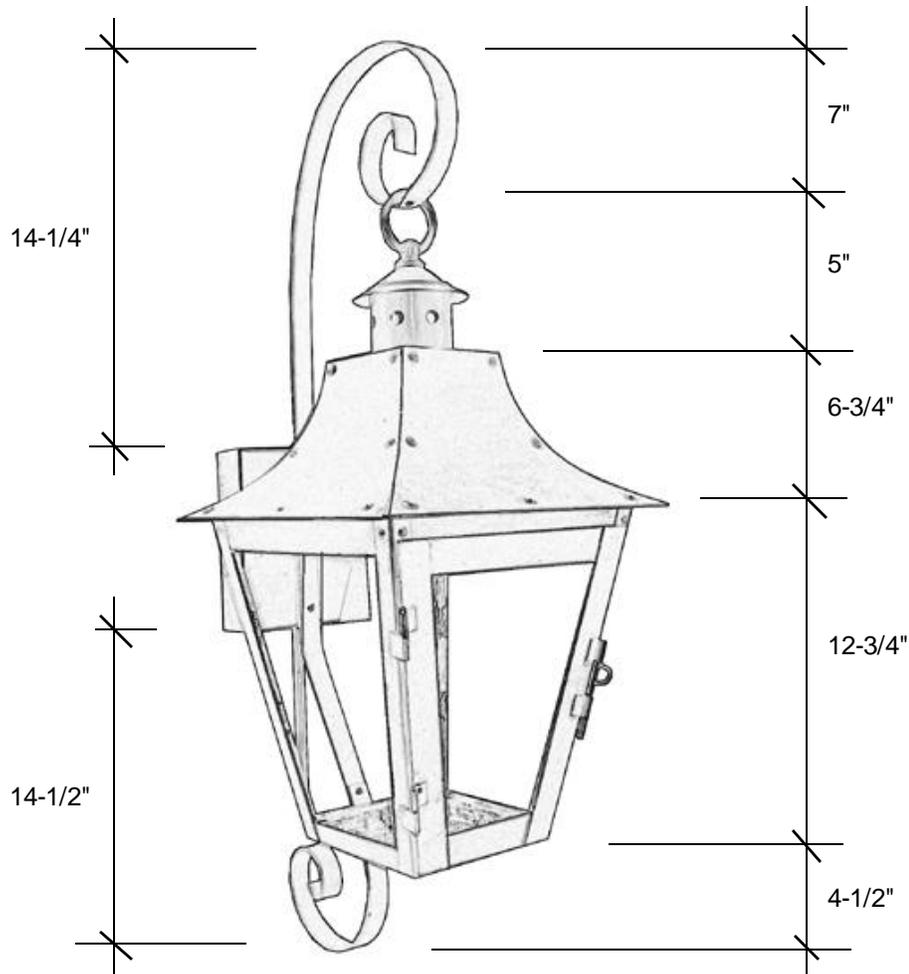
This fixture is available with clear glass only and comes standard with natural gas components with an option of propane. The fixture has a manual on/off valve with a maple leaf design and has a BTU rating of 3011. Electronic starters are not available.
