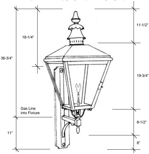
This fixture is available with clear tempered glass only and is listed for natural gas, with an option of propane. The fixture has a manual on/off valve with a maple leaf design and has a BTU rating of 3011.
