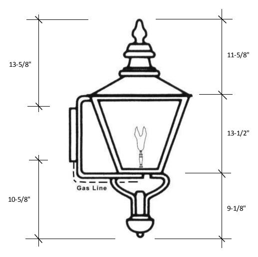
This fixture is available with clear tempered glass only and is UL listed for natural gas, with an option of propane. The fixture has a manual on/off valve with a maple leaf design and has a BTU rating of 3011.
