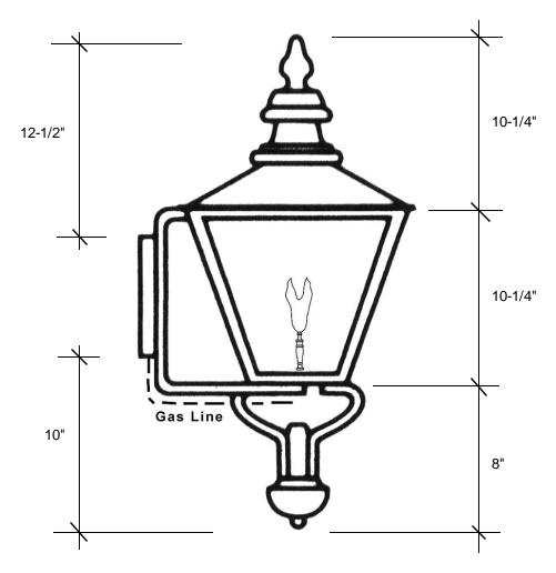
This fixture is available with clear tempered glass only and is UL listed for natural gas, with an option of propane. The fixture has a manual on/off valve with a maple leaf design and has a BTU rating of 3011.
